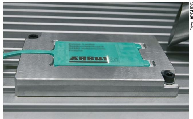
Laser marking of silicone with color change
