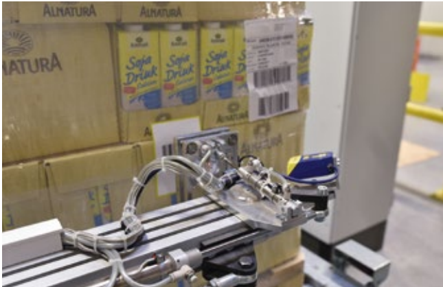
Pallet labeling at various heights
