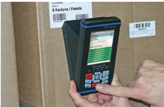
Flexible verification of barcodes on site
