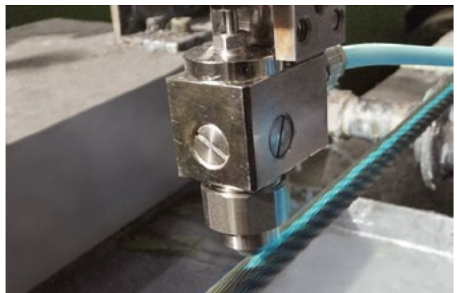
Color marking of wire cables
