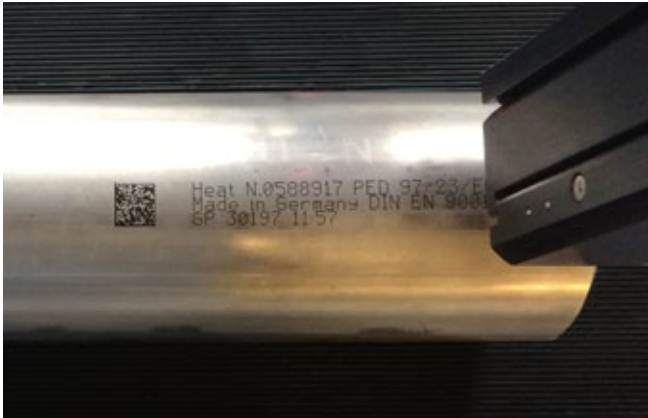
Coding and marking of steel pipes
