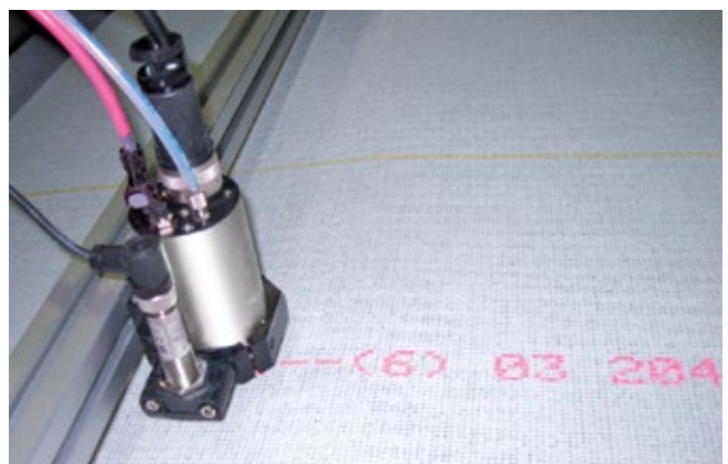
Coding and marking of sheeting materials
